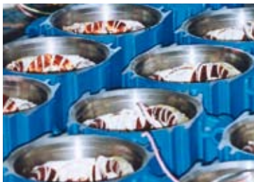
Electrical winding (stator) pressed in the motor casing
