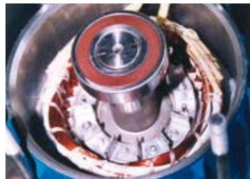
Stator (electrical winding) and rotor at GTWS
