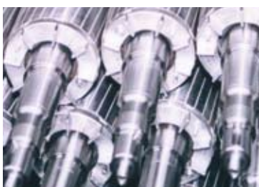
Rotor pressed on shaft
