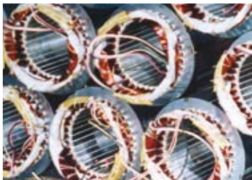
Electric winding (stator of laminations with three-phase winding)
